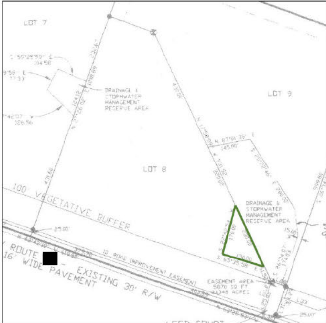
Drainage & Stormwater Management Area
